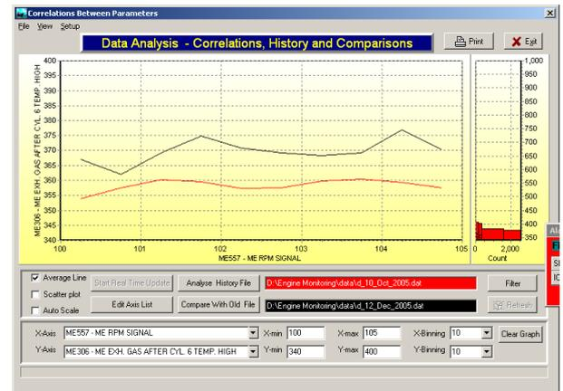
Fig. 10: Mean exhaust gas temp, filtered by draught.
