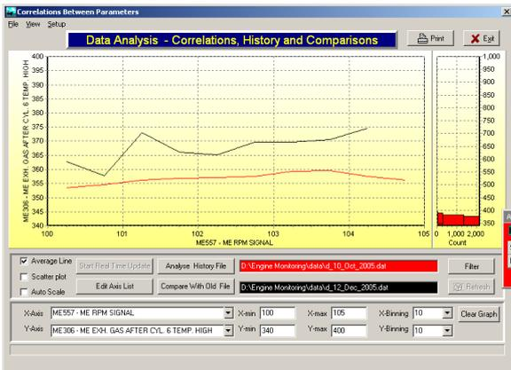
Fig. 11: Mean exhaust gas temp, filtered by draught and sea water temperature.
