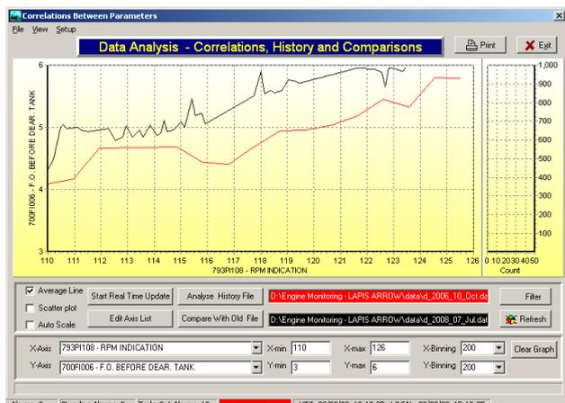
Fig. 9: Fuel consumption, filtered by draught.
