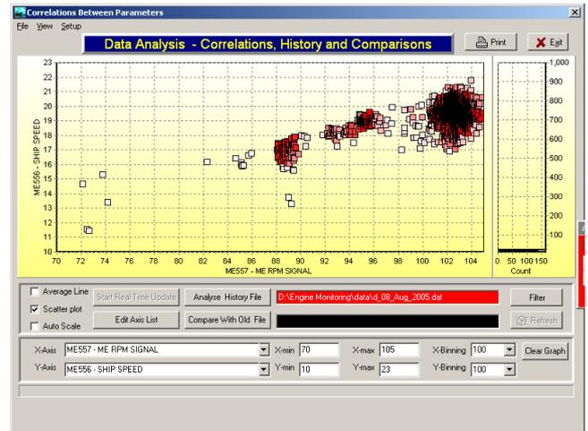
Fig. 4: Speed vs. RPM, with filter on draft – greater than 8.5 meters.
