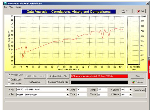
Fig. 7: Speed vs. RPM, average value, with filter on draft – greater than 8.5 meters.
