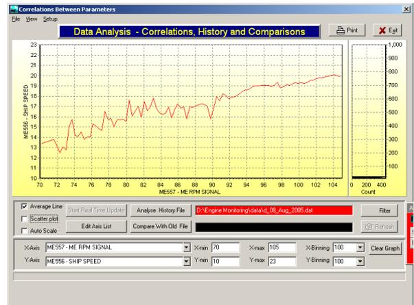
Fig. 6: Speed vs. RPM, average value, no Filter
