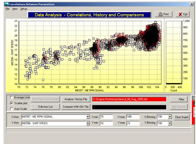
Fig. 3: Speed vs. RPM, no Filter
